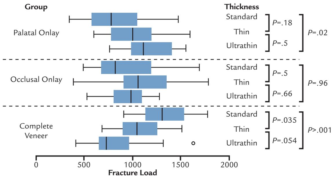
**4** Box plots of single load to failure test results in newtons (N). Comparison of groups with identical preparation design and different ceramic thicknesses.
