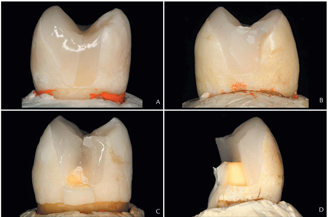
**5** Representative photographs of failed specimens in proximal view. A, I: Extensive crack formation within ceramic. B, II: Cohesive fracture within ceramic. C, III: Fracture within ceramic and tooth structures. D, IV: Longitudinal ceramic and tooth fracture involving root.
