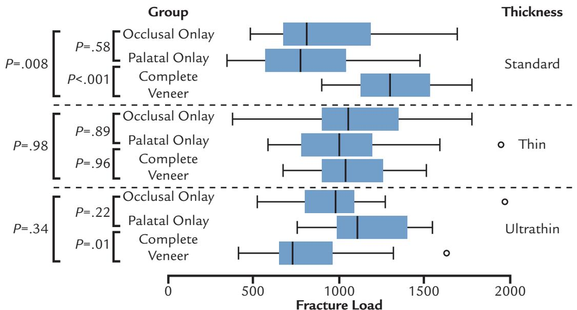
**3** Box plots of single load to failure test results in newtons (N). Comparison of groups with identical ceramic thickness and different preparation designs.
